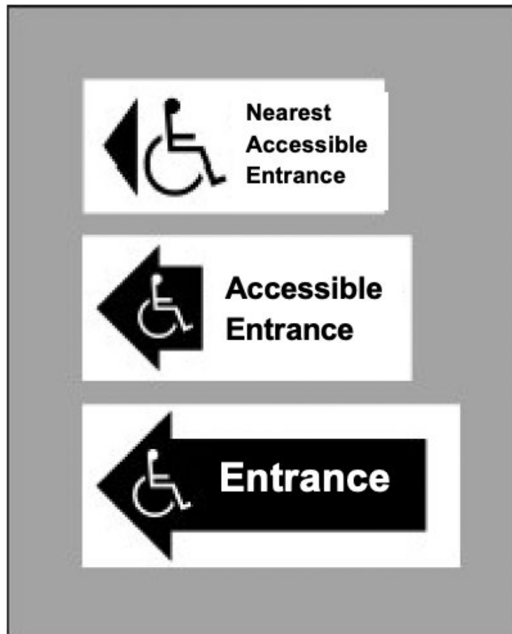
Figure 48: ISA signs directing individuals to the accessible route to a polling place.
